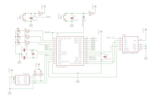
A reset button pulls MCLR to ground when pressed, with C2 designed to prevent debounce noise. D1 prevents programming voltages on MCLR/VPP reaching the +5V buss. C3, C4 and crystal allow the PIC to run at 64Mhz (via the PLL), or 16mips. C1 is a power supply bypass for the PIC.
