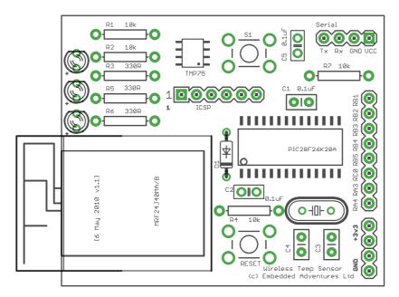
The board is designed to allow you to construct the entire project by hand soldering. Even the surface mount parts are not difficult. Please see the "Building Kits" section under Tutorials on the EA web site – www.embeddedadventures.com – for more information.
